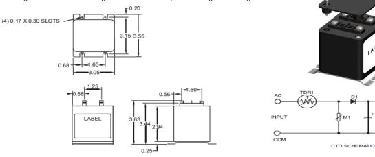
These devices are protected against inadvertent short circuits, input from line surges and inductive kickback from trip coils.
