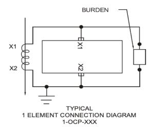
The single element Open Circuit Protector is provided with two terminals for connection across the secondary of the C.T. and in parallel with burden. It can also be connected across the current terminals of a protective relay, meter, or other current operated device without affecting the operation of the device. Secondary polarity of the C.T.'s is not critical to the OCP.
